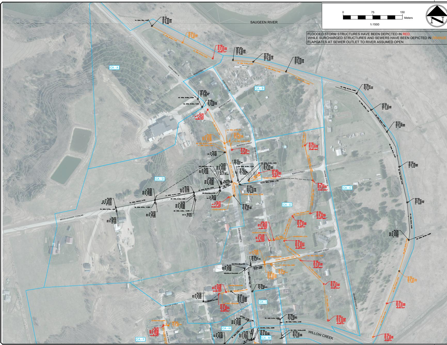
FLOODED STORM STRUCTURES HAVE BEEN DEPICTED IN **RED**, WHILE SURCHARGED STRUCTURES AND SEWERS HAVE BEEN DEPICTED IN **ORANGE**. FLAPGATES AT SEWER OUTLET TO RIVER ASSUMED OPEN
