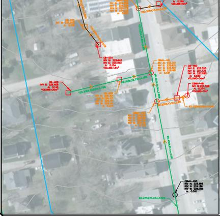
FLOODED STORM STRUCTURES HAVE BEEN DEPICTED IN RED, RECOMMENDED STORM STRUCTURES HAVE BEEN DEPICTED IN GREEN, WHILE SURCHARGED STRUCTURES AND SEWERS HAVE BEEN DEPICTED IN ORANGE FLAGGATES AT SEWER OUTLET TO RIVER ASSUMED OPEN.
