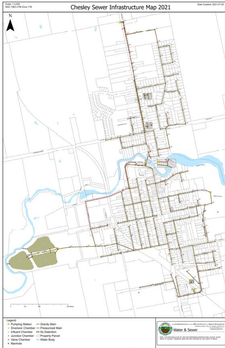
Sanitary Sewer System Map – Chesley
