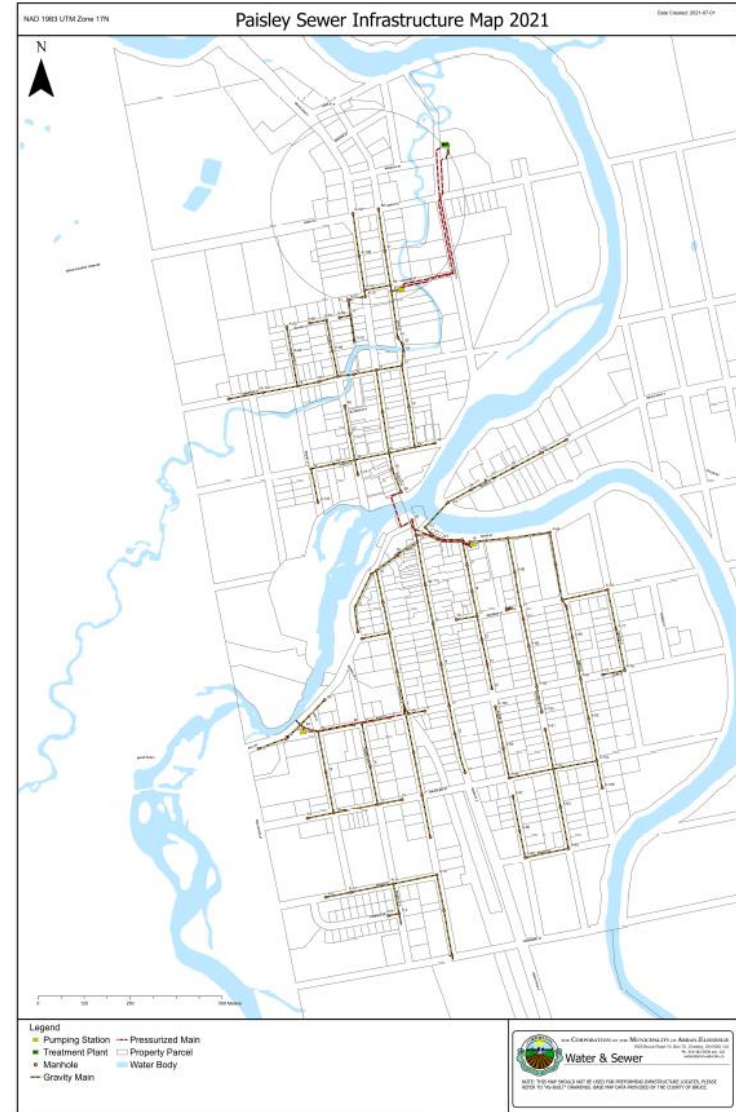
Sanitary Sewer System Map – Paisley
